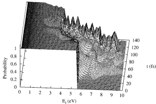
**Figure 5.** Evolution of the occupation probability  $f(E_i)$  in the metal film during the interaction with a femtosecond laser pulse with photon energy  $\hbar\omega = 1.55$  eV and peak intensity  $I_0 = 10^{12}$  W cm $^{-2}$ . During the laser interaction, increasing oscillations of the occupation of states in the energy domain appear, leading to an inversion of states (cf figure 4 and text).
