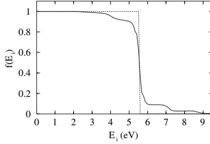
**Figure 1.** Occupation probability of states in a metal film of thickness  $L = 32$  nm after a short laser pulse of duration 17.34 fs (solid curve), starting from the initial distribution at zero temperature (dotted curve). The interaction with laser photons of energy  $\hbar\omega_0 = 1.55$  eV at peak intensity  $I_0 = 10^{12}$  W cm $^{-2}$  leads to a step-like occupation of states above the Fermi energy  $E_F = 5.51$  eV (workfunction  $W = 4.3$  eV) by one- and two-photon absorptions.
