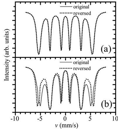
Fig.1. Simulation of reciprocity-obeying (a) and violating (b) arrangements in Mössbauer scattering [MR.1].
