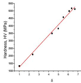
*Fig. 2. Hardness versus  $\delta$  for single-phase HEA's*
