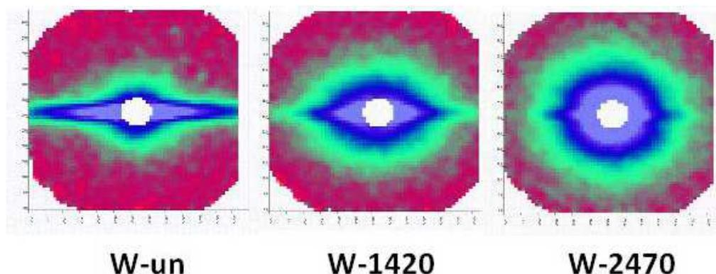
Fig.2. 2D SANS scattering intensities of the 0.5 mm diameter tungsten samples taken from the different steps of the wire production. Temperatures of annealing: not annealed, 1420 K and 2470 K
