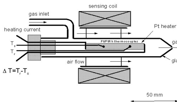
Fig.4. Probe head for DTA and TMAG measurements
