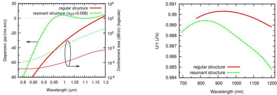
Fig. 2 Computed dispersion and confinement loss(left) and computed stored energy-group delay ratio (right) in solid core PBG fibers of two different designs having a unit length of 1 m (incident power is 1W).
