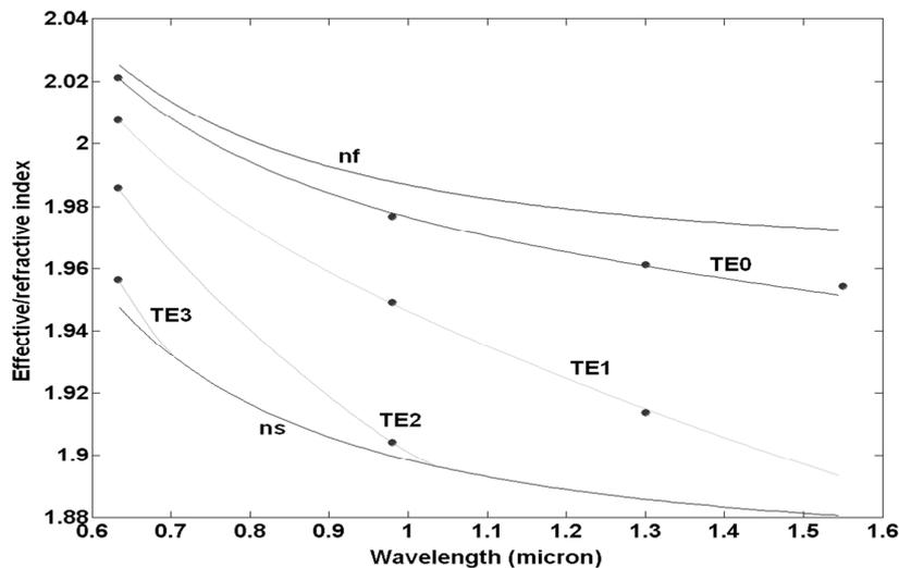
Fig.2. Multispectral reconstruction of the refractive index of the guiding and barrier layer as a function of the wavelength in a 3.5 MeV  $\text{N}^+$  ion irradiated planar waveguide in Er: Te glass. Sample was irradiated with  $8 \times 10^{16}$  ions/cm $^2$ . Calculated effective indices (nf and ns) of the modes are also shown.
