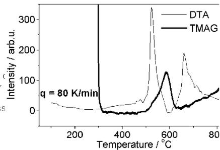
Fig.5. DTA and TMAG crystallization patterns.
