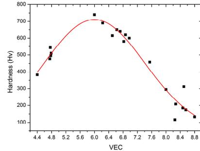
*Fig. 3. Hardness versus VEC for single-phase HEA's*
