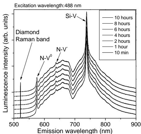
Fig. 2 Photostability of color centers in nanodiamond at power density of 12 kW/cm<sup>2</sup>.
