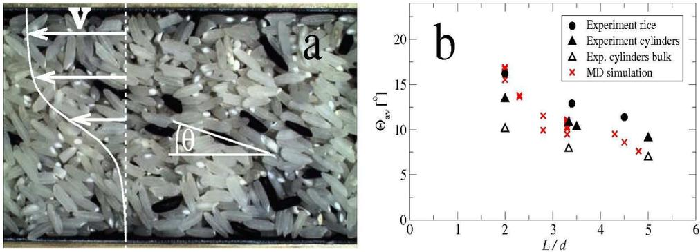
Fig. 2. (a) Shear induced alignment of elongated grains; (b) the alignment angle decreases with increasing particle length.
