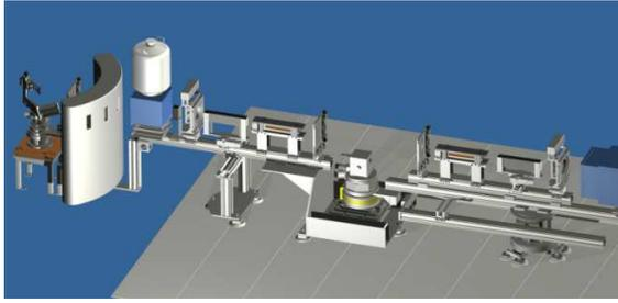
Figure 2. Layout of the GINA neutron reflectometer with the upgraded monochromator and slits
