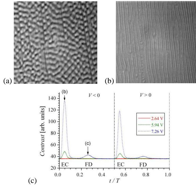
Fig. 1. (a) EC pattern; (b) flexoelectric domains; (c) pattern contrast vs. time at 30 mHz.
