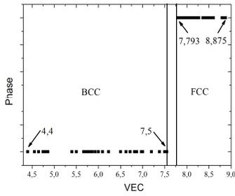
*Fig. 1. Crystallographic phase versus VEC for single-phase HEA's*
