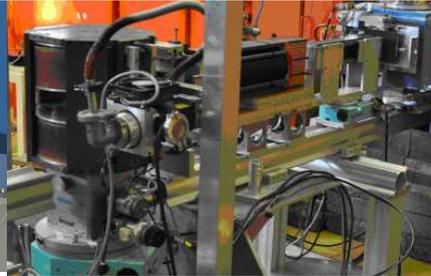
Figure 3. The installed low temperature sample environment of the GINA reflectometer
