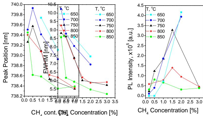
Fig. 1 Evolution of Si-V photoluminescence peak parameters with methane content of the feed gas in sample sets prepared at different substrate temperatures.
