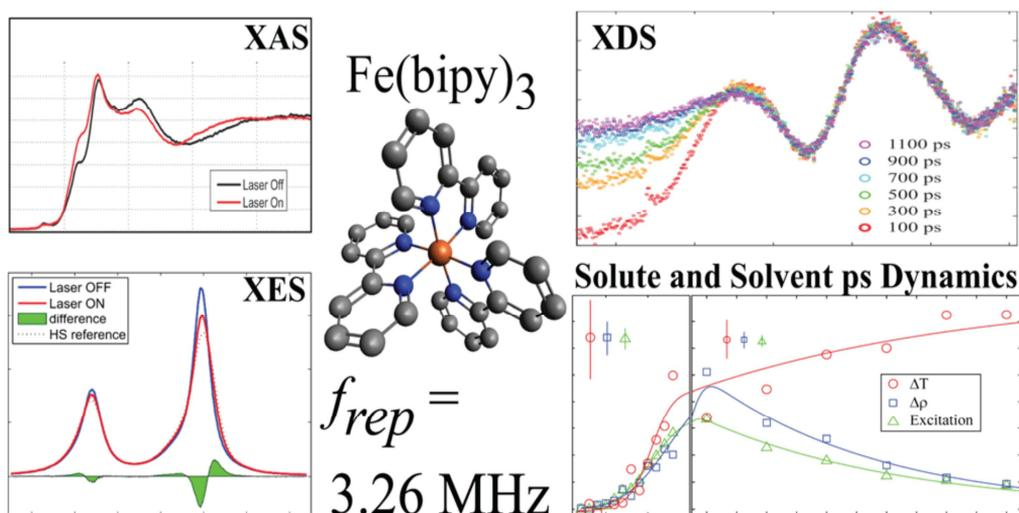
**Fig. 1.** Combined X-ray absorption and X-ray emission spectra, and X-ray diffuse scattering results that resolve a subnanosecond-lived excited Fe(II) state.
