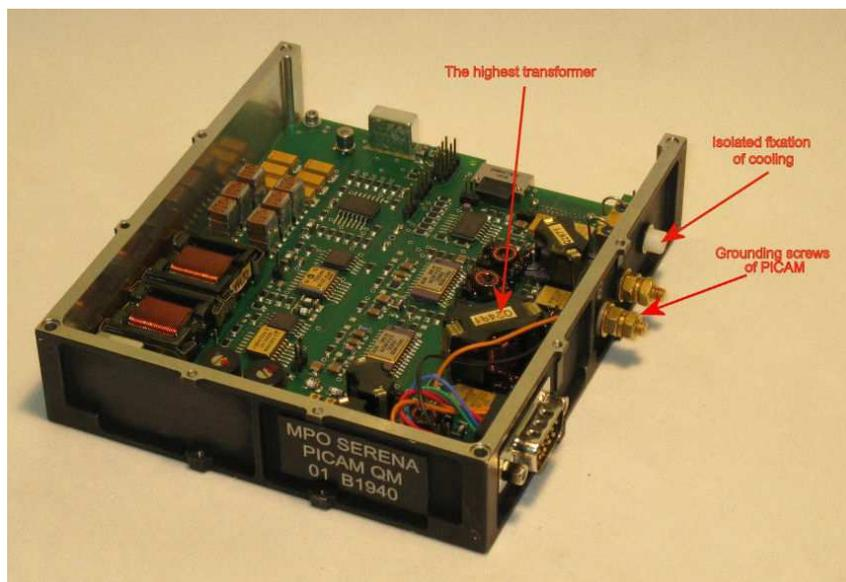
*Fig 1. The Qualification Model of the DCC for the PICAM instrument*
