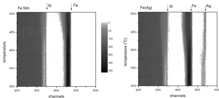
*Fig. 1. Real-time BS measurements using 2000 keV  $^4\text{He}^+$ -beam on a 50 nm Fe film (left) and Fe film containing 1 at. % Ag (right) on Si(100) using ramped annealing (1.9 °C/min). Every horizontal line in such a contour plot corresponds to an RBS spectrum, with a tone scale representing the backscattering yield.*
