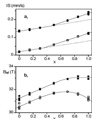
Fig. 2. Average isomer shift (a) and hyperfine field (b) of  $\text{Co}_2\text{FeAl}_{1-x}\text{Si}_x$  measured at room temperature (empty circles) and at 12 K (dots).
