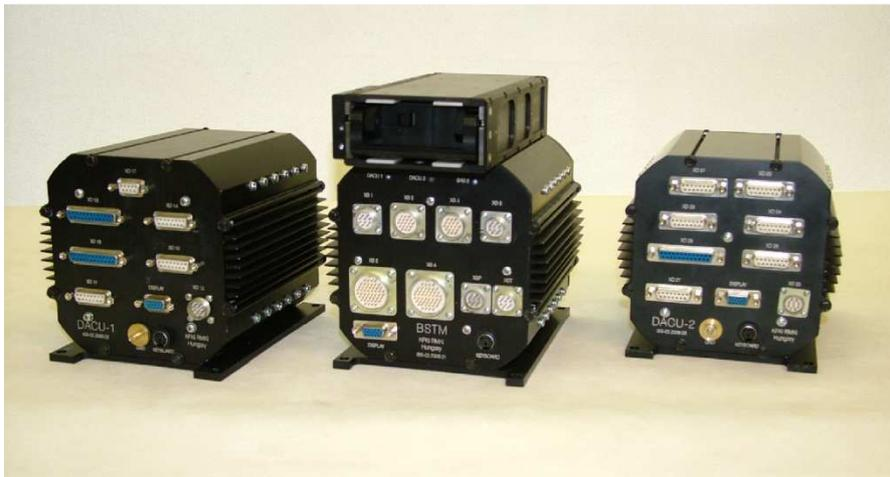
Fig. 2. The distributed computer system of the Obstanovka
