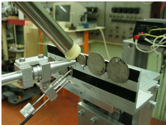
Figure 3. Ancient silver coins fixed to the positioning device. The beam pipe- detector arrangement and the mechanical aiming tool of the external beam PIXE set-up can also be seen.
