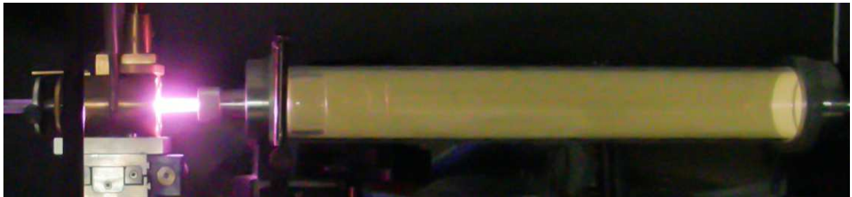
Figure 5. Microwave surface-wave excited plasma (left, bright part), and reactive streaming afterglow (right, large volume part)
