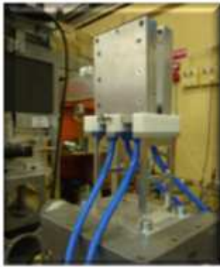
Figure 2. The new biomembrane option for the GINA neutron reflectometer
