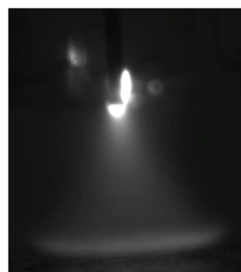
Figure 2.b. The structure of the visible glow of the plasma needle.
