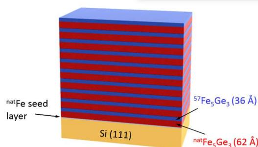
**Figure 1.** Layer structure of Fe<sub>5</sub>Ge<sub>3</sub> isotope periodic multilayer structure.
