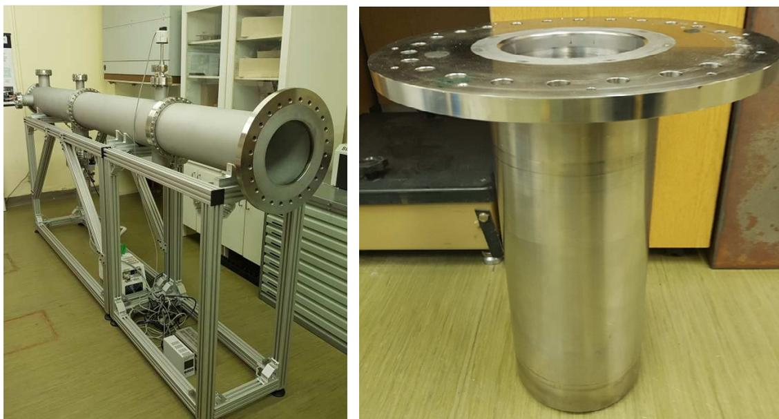
**Figure 3.** Left: Vacuum chamber for the testing of the JT-60SA video diagnostic port plug for EDICAM. Right: Mock-up port plug.
