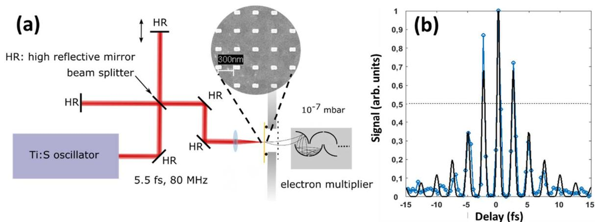
**Figure 1.** (a) The output of an interferometric autocorrelator setup illuminated by 5.5-fs laser pulses is focused onto a substrate with plasmonic nanoparticles. Photoelectron spectra are recorded in vacuum. (b) Measured (blue) and reconstructed (black) third-order interferometric autocorrelation curves of the few-femtosecond plasmonic near-field.
