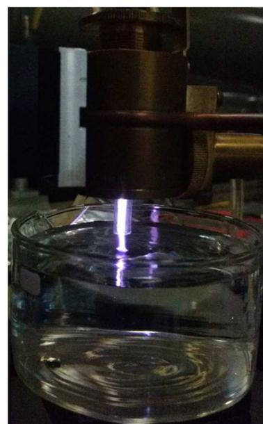
**Figure 5.** A surface-wave microwave discharge in interaction with water surface.
