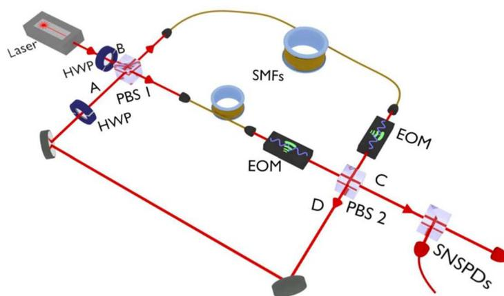
**Figure 2.** Schematic of the experimental setup of the time-multiplexed quantum walk with active in- and outcoupling realized by two EOMs (electro-optical modulators). The active control of the switches allows to implement in the time domain both the continual and reset measurement schemes. HWP, half-wave plate; PBS, polarizing beam splitter; SMF, single-mode fiber; SNSPDs, superconducting nanowire single-photon detectors.
