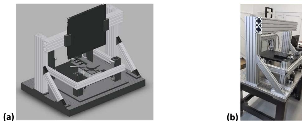
**Figure 2.** Design (a) and realization (b) of the confocal microscope stand.
