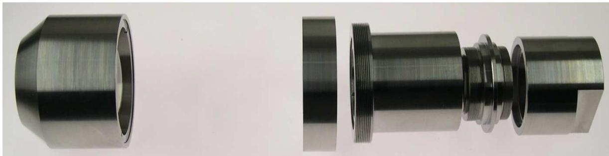
**Figure 2.** Optics in stainless steel housing for the JT-60SA EDICAM diagnostic.
