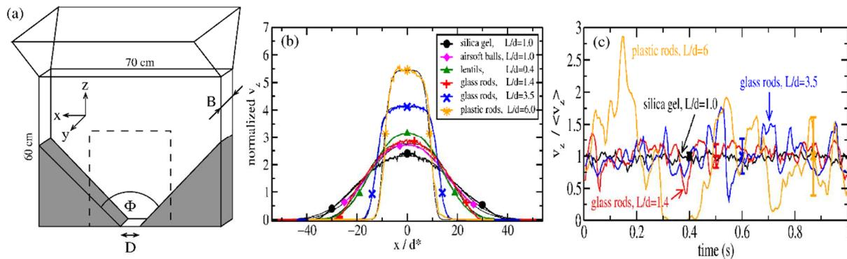
**Figure 1.** (a) Sketch of the quasi-two-dimensional hopper, (b) vertical velocity across the hopper, (c) time evolution of the vertical velocity.
