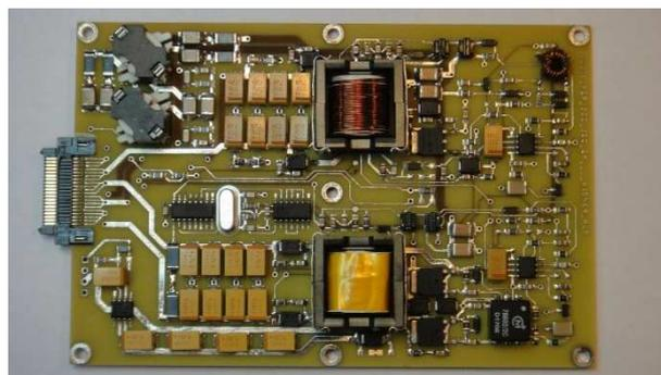
**Figure 2.** DCC for JDC sensor.
