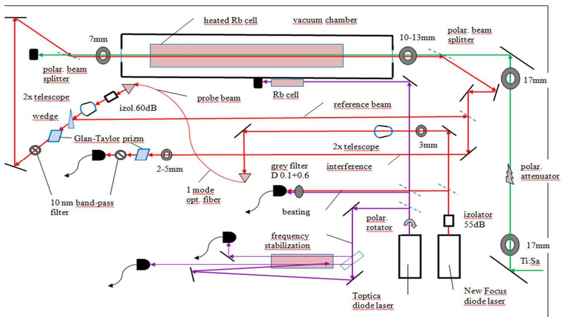
Fig.1. The scheme of the real-time interferometric diagnostic scheme.
