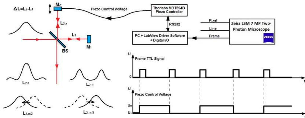
**Figure 1.** A Michelson-interferometer is used for spectral modulation of the pump pulses. Depending on the electronically controlled phase difference of the two arms, different spectra can be generated for CARS imaging.  $\Delta L$  has a properly set offset value depending on the spectral bandwidth of the laser applied. The phase difference is electronically controlled and synchronized to the frame signal of our microscope.
