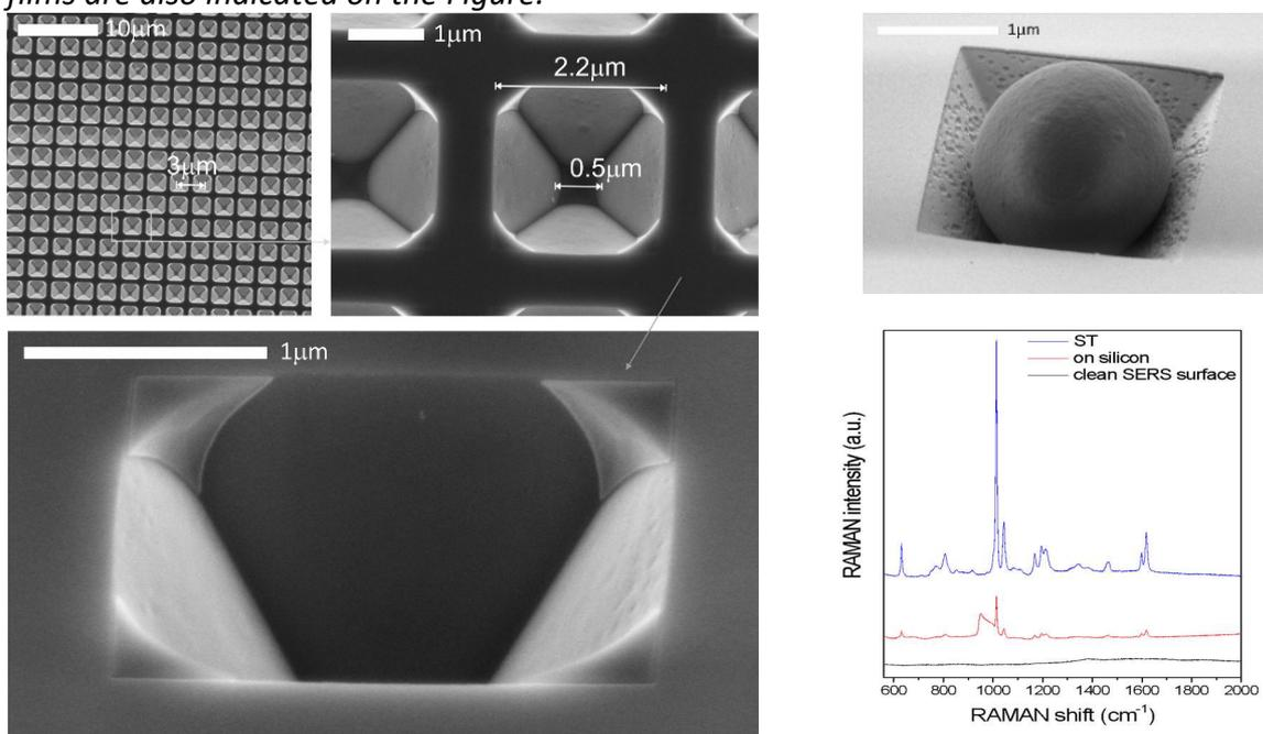
**Figure 2.** SEM view of the periodic perforated SERS substrate applicable for flow-through experiments and particle and cell entrapment (left). Polymeric microparticle entrapped in an inverse pyramid of the SERS substrate (top right). Comparison of the SERS spectra recorded on the clean SERS surface and entrapped microparticle (ST) and normal Raman spectrum of the latter on silicon (bottom right).
