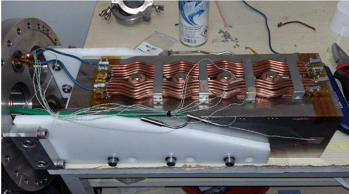
**Figure 2:** ITER VV mockup-segment with the installed loom elements
