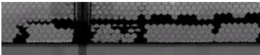
Fig.3. Honeycomb structure of a helicopter rotor blade section (90×30 cm 2 ) with an extensive water percolation (dark areas) as revealed by neutron radiography
