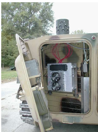
Fig 1. Intelligent Laser Warner System installed on the vehicle
