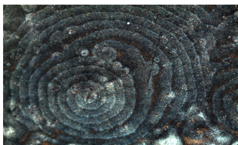
Figure 1. Spiral structure on the surface of electrodeposited Ag-Sn alloy.
