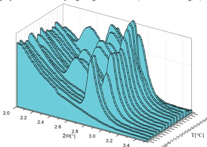
**FIGURE 4.** Low angle segment of X-ray diffractograms of **M2** at different temperatures
