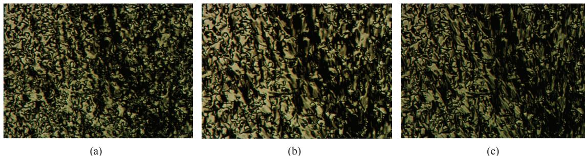
**FIGURE 3.** Micrographs of **M2** in: (a) nematic phase at 87°C, (b) smectic SmA phase at 80°C and (c) SmC phase at 73°C
