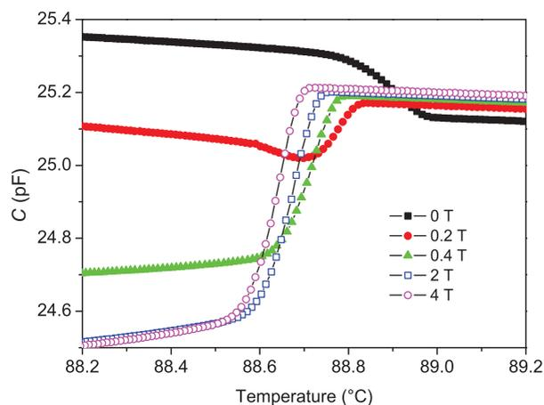
Figure 4. (colour online) Capacitance versus temperature for the liquid crystal mixture doped with spherical  $\text{Fe}_3\text{O}_4$  MNPs for different values of the magnetic induction.
