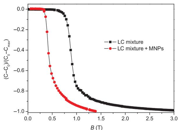
Figure 2. (colour online) Relative capacitance versus magnetic induction for the liquid crystal mixture and for the liquid crystal mixture doped with spherical  $\text{Fe}_3\text{O}_4$  MNPs at  $T = 80^\circ\text{C}$ .
