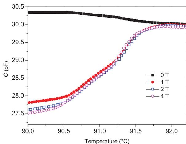
Figure 3. (colour online) Capacitance versus temperature for the undoped liquid crystal mixture for different values of the magnetic induction.
