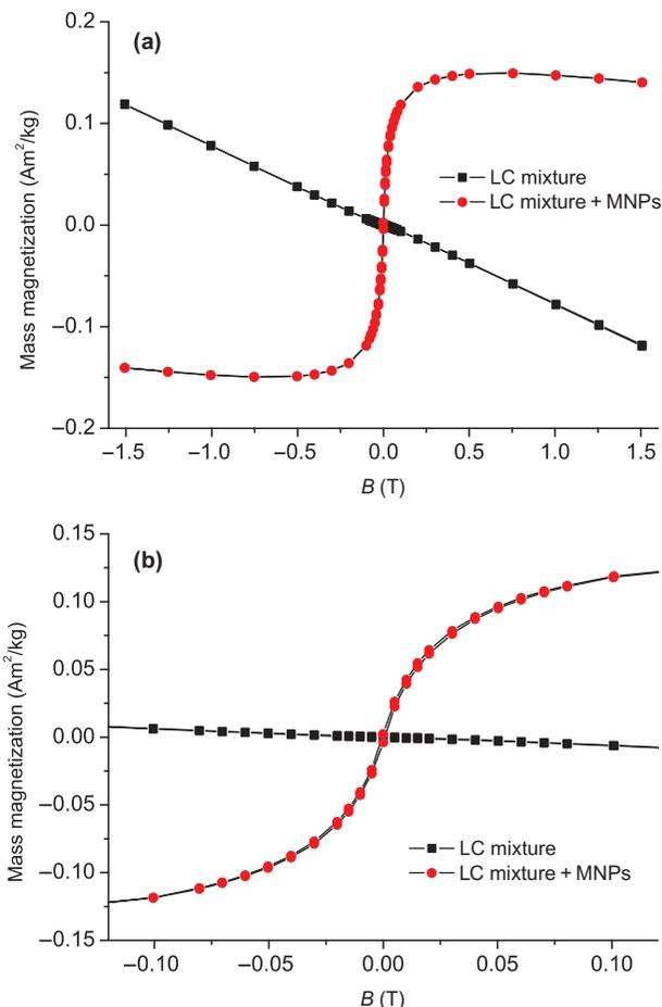
Figure 1. (colour online) (a) Magnetisation curves of the LC mixture and the LC mixture doped with magnetic particles (MNPs), measured at  $T = 80^\circ\text{C}$ . (b) A blow-up of the magnetisation curves around zero magnetic field.
