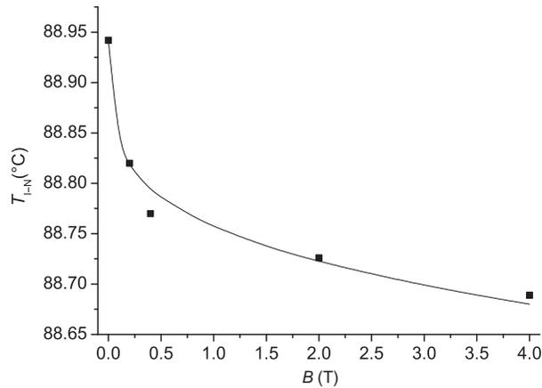
Figure 5. The isotropic–nematic phase transition temperature versus the applied magnetic induction, measured in the liquid crystal mixture doped with spherical magnetic nanoparticles. Size of the symbols corresponds to the uncertainty of the measurements. The solid curve corresponds to a fit to Equation (1).
