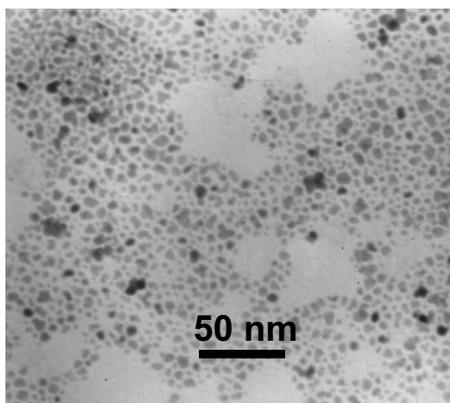
FIG. 1. TEM image of spherical magnetic particles.
