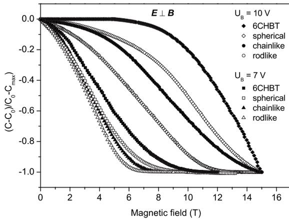
FIG. 10. Reduced capacitance dependence of pure 6CHBT and 6CHBT doped with spherical, chainlike, and rodlike particles on external magnetic field measured at  $U_B=7$  V and  $U_B=10$  V.
