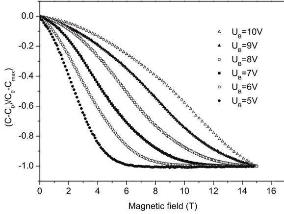
FIG. 8. Reduced capacitance dependence of 6CHBT doped with rodlike particles on external magnetic field measured at different bias voltages.
