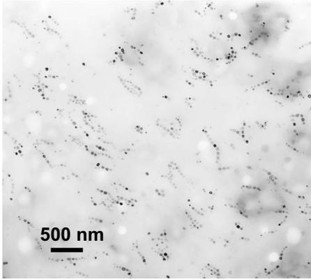
FIG. 5. TEM image of chainlike magnetic particles.
