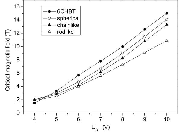
FIG. 9. Dependence of critical magnetic field on the bias voltage for pure 6CHBT and 6CHBT doped with spherical, chainlike, and rodlike particles.
