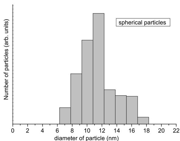
FIG. 2. Histogram of size distribution of spherical magnetic particles.
