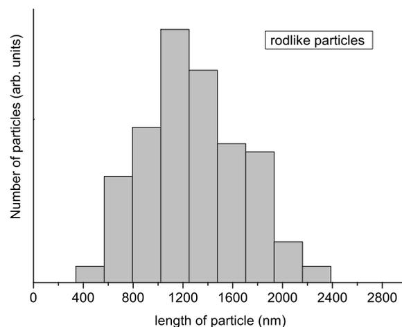
FIG. 4. Histogram of length distribution of rodlike magnetic particles.
