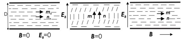
FIG. 7. Cross section of the cell in the initial state, after application of the electric field  $E_B > E_C$  and after application of the external magnetic field  $B > B_C$ .
