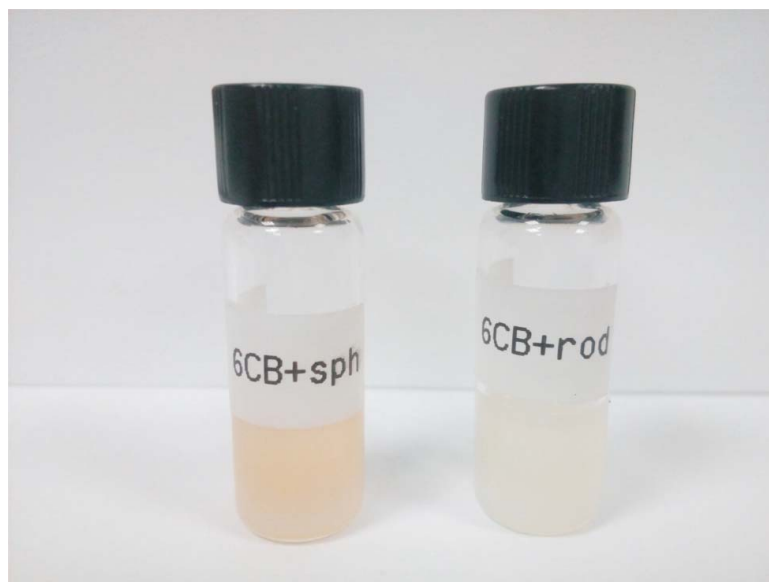
Figure 1. Pictures of ferronematics with spherical (left-hand side), and with rod-like (right-hand side) MNPs, taken about three months after the preparation.
