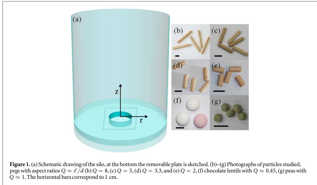
**Figure 1.** (a) Schematic drawing of the silo, at the bottom the removable plate is sketched. (b)–(g) Photographs of particles studied, pegs with aspect ratios  $Q = \ell/d$  (b)  $Q = 8$ , (c)  $Q = 5$ , (d)  $Q = 3.3$ , and (e)  $Q = 2$ , (f) chocolate lentils with  $Q \approx 0.45$ , (g) peas with  $Q \approx 1$ . The horizontal bars correspond to 1 cm.
