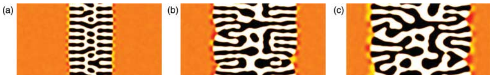
Figure 32. Snapshots of eutectic solidification on the atomistic scale in the binary 1M-PFC model in 2D [28]: composition \hat{\psi} maps corresponding to 2 \times 10^5 , 6 \times 10^5 , and 10^6 time steps are shown. White and black denote the two crystalline phases, while grey (orange online) stands for the liquid phase. The simulation has been performed on a 2048 \times 1024 rectangular grid. Crystallization has been started by placing a row of supercritical crystalline clusters of alternating composition into the simulation window. Interestingly, the eutectic pattern evolves inside the solid region on a timescale comparable to the timescale of solidification. (Reproduced from Tóth et al. [28] © 2010 by Institute of Physics Publishing.)
