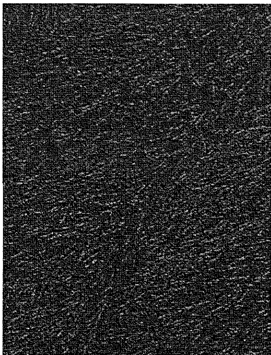
Figure 1. Texture of the most stable, regular crystal form of a 10 \mu\text{m} thick film of 8OCB.
