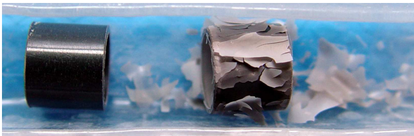
FIG. 7 View of E110G (left) and E110 (right) cladding samples after 5000 s oxidation at 900°C in steam.
