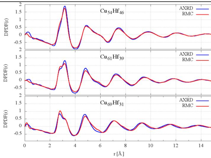
**Figure 3.** Comparison of Hf differential pair distribution function  $DPDF_{Hf}(r)$  extracted by AXRD and from the 3D RMC configuration box.
