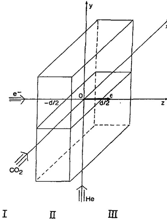
**Figure 1.** This figure shows the geometry of the intersection of the atomic beam of rectangular cross section, propagating in the  $y$  direction, with the electron beam, propagating in the  $z$  direction, and the laser beam, propagating in the  $x$  direction, having its vector of linear polarization parallel to the  $z$  axis.
