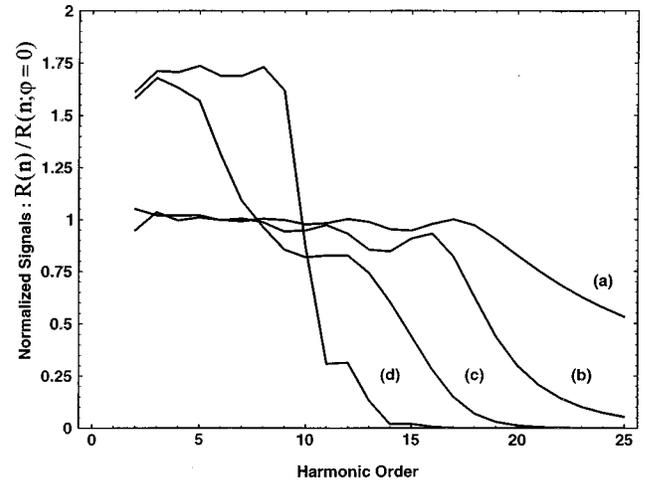
FIG. 3. Demonstrates more drastically the increase of  $R_n/n$  at small  $n$  by presenting  $R_n(\varphi)/R_n(\varphi=0)$  for (a)  $\varphi=\pi/4$ , (b)  $\varphi=\pi/2$ , (c)  $\varphi=3\pi/4$ , and (d)  $\varphi=\pi$ . Simultaneously one recognizes the decrease of the cutoff frequency.
