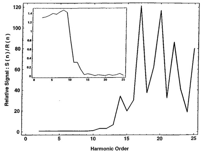
FIG. 4. Shows on a large scale  $S_n/R_n(\varphi=\pi)$  and in the inset  $R_n(\varphi=\pi)/S_n$ , where  $S_n$  are the rates for a single frequency. While the inset drastically demonstrates the early cutoff of the spectrum for  $\varphi=\pi$ , the large scale figure shows for higher  $n$  the zigzagging of the harmonic rates for  $\varphi=\pi$  which are already apparent in Fig. 1.
