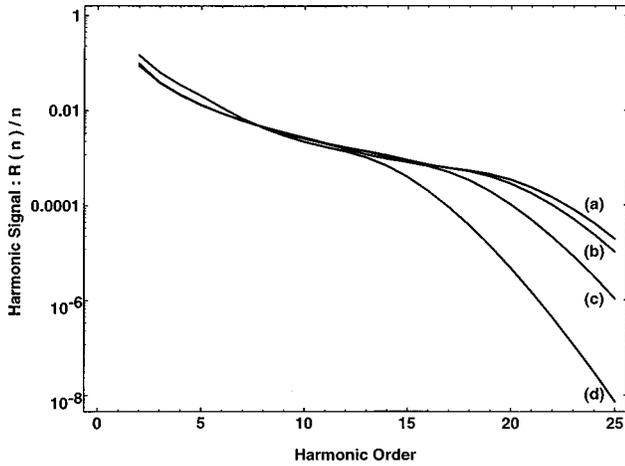
FIG. 2. Shows the decrease of the number of harmonics generated with increasing  $\varphi$  for (a)  $\varphi=0$ , (b)  $\varphi=\pi/4$ , (c)  $\varphi=\pi/2$ , and (d)  $\varphi=3\pi/4$ . Here too one recognizes the features already apparent in Fig. 1, such as the enhancement of the harmonic rates for small  $n$  with increasing phase  $\varphi$ .
