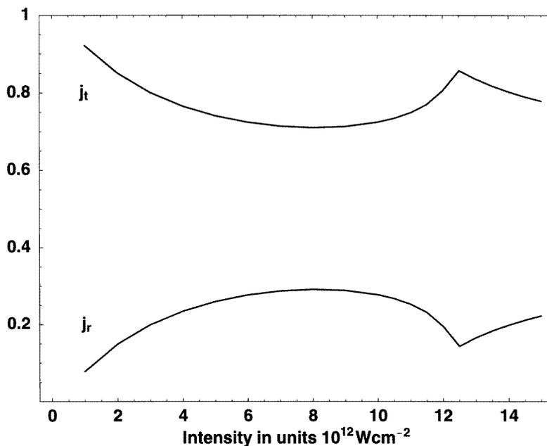
**Figure 2.** The total transmitted and reflected currents,  $j_t$  and  $j_r$ , respectively, as a function of the laser intensity  $I$ . If the initial kinetic energy of the electron in the laser field is chosen  $E'_{\text{kin}} = 0.05$  eV, then at the particular intensity of  $1.25 \times 10^{13}$  W cm $^{-2}$  a *cusp* appears due to the opening of a further channel at  $n = -1$ .
