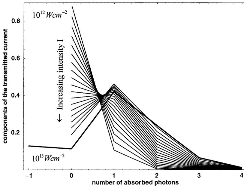
**Figure 1.** If the initial electron kinetic energy in the laser field is chosen as  $E_{\text{kin}}^i = 0.28$  eV, the transmitted current components,  $j_t(n)$ , are shown as a function of the number of absorbed photons  $n$ . With increasing intensity  $I$  of the laser field,  $j_t(0)$  is decreasing and, at the same time,  $j_t(1)$  is gradually increasing, while at an intensity of  $10^{13}$  W cm<sup>-2</sup> the channel with  $n = -1$  gets opened.
