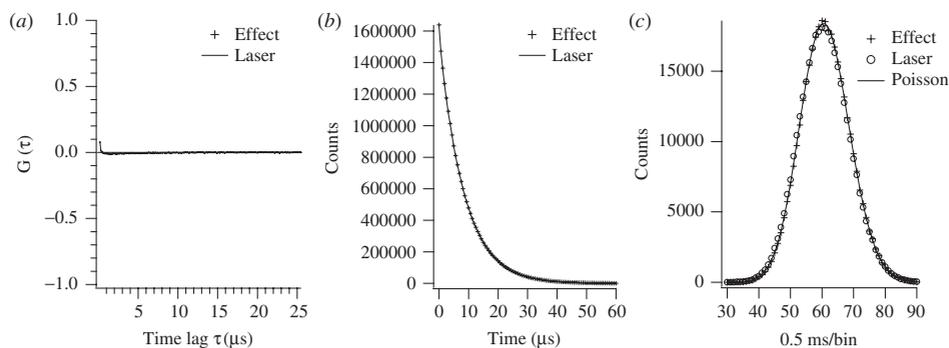
Figure 5. Correlation function (a), time interval distribution between the neighbouring photons (b) and the number distribution of the detected photons in definite (preset) sampling time (c) of the exciting laser beam (laser) and the light emitted by generated plasmons (effect).
