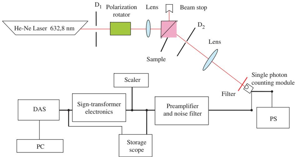
Figure 4. Experimental set-up for measurement of photon statistics of surface plasmons. (The colour version of this figure is included in the online version of the journal.)
