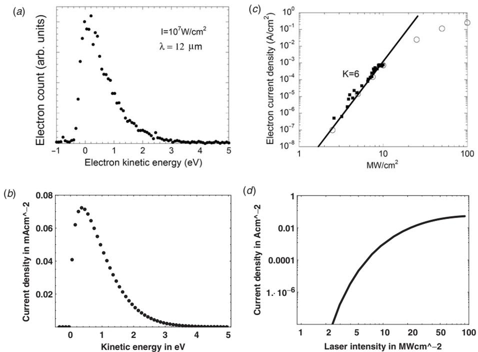
Figure 2. Experimental (a) and theoretical (b) photoelectron spectra at  $100 \text{ MW/cm}^2$  laser intensity and 12 microns wavelength and the intensity dependence of the total photocurrent density according to the experiment (c) and the present theory (d).
