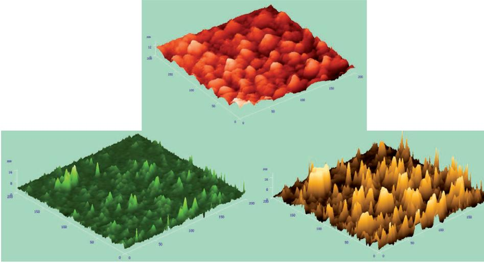
Figure 1. Simultaneously measured topographic, surface plasmon EM field and thermal images obtained by an STM. (The color version of this figure is included in the online version of the journals.)
