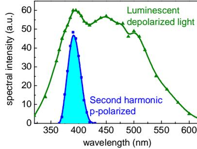
Fig. 3. Second harmonic (blue solid line) and continuum (green solid line) spectra scattered from the metal surface upon SPP excitation with 795-nm, 120-fs pulses.
