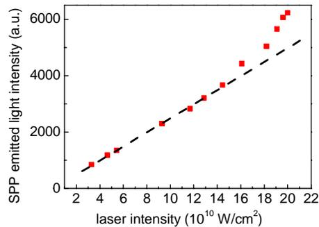
Fig. 2. Intensity dependence of the SPP-emitted light with femtosecond SPP excitation (squares). Nonlinear deviation from the linear fit to the first points (dashed line) starting at  $1.4 \times 10^{11}$  W/cm<sup>2</sup> focused intensity is observed.
